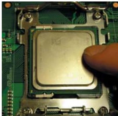
4. With the CPU inserted into the socket, inspect the four corners of the CPU to make sure that it is properly installed and flush with the socket. Then, gently lower the silver CPU retention plate into place.
