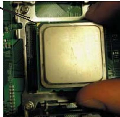
3. Align pin 1 of the CPU with pin 1 of the socket. Once aligned, carefully place the CPU into the socket. *Do not drop the CPU on the socket, move the CPU horizontally or vertically or rub the CPU against the socket or against any pins of the socket, which may damage the CPU and/or the socket.*
