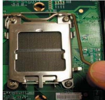
2. Use your thumb and your index finger to hold the CPU. Locate and align pin 1 of the CPU socket with pin 1 of the CPU. Both are marked with a triangle.
