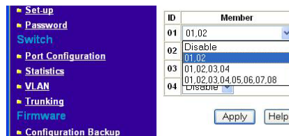
Figure 5-5. Switch> Trunk Setting: Trunk Group 01
