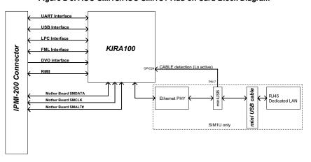
The block diagram for the AOC-SIM1U/AOC-SIM1U+ add-on card is shown in Figure 2-5.
