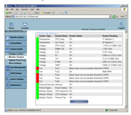
Figure 3-11. Monitor Sensor Screen
