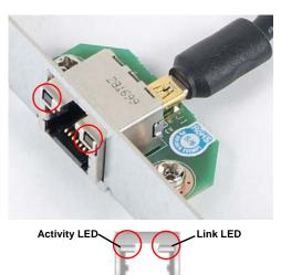
There are two LAN LED Indicators located on the (Dedicated) LAN port on the AOC-USB2RJ45 Add-On Card (see Figure 2-4). The green LED indicates activity, while the power LED may be green or off to indicate the speed of the Ethernet connection. See Table 2-4 for more information.
