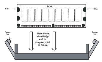
Note the notch in the slot and on the bottom of the DIMM. These prevent the DIMM from being installed incorrectly.
