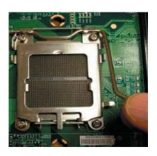
2. Use your thumb and your index finger to hold the CPU. Locate and align pin 1 of the CPU socket with pin 1 of the CPU. Both are marked with a triangle.
