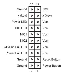
Figure 2-4. JF1: Front Control Panel Header (JF1)
