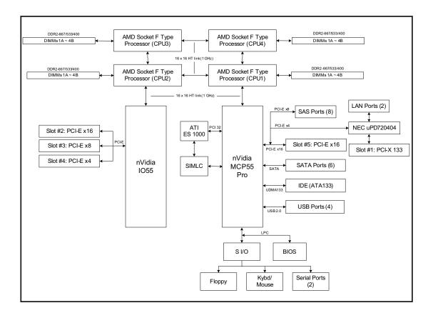
Figure 1-3. nVidia MCP55 Pro/IO55 Chipset: System Block Diagram
