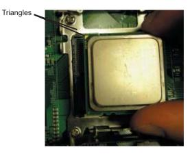
3. Align pin 1 of the CPU with pin 1 of the socket. Once aligned, <u>carefully</u> place the CPU into the socket. Do not drop the CPU on the socket, move the CPU horizontally or vertically or rub the CPU against the socket or against any pins of the socket, which may damage the CPU and/or the socket.
