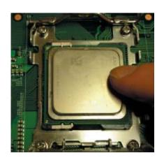
4. With the CPU inserted into the socket, inspect the four corners of the CPU to make sure that it is properly installed and flush with the socket. Then, gently lower the silver CPU retention plate into place.
