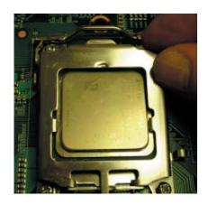
5. Carefully press the CPU socket lever down until it locks into its retention tab. For a dual-CPU system, repeat these steps to install another CPU into the CPU#2 socket (and into CPU#2, #3 and #4 sockets for a quad-CPU configuration).
