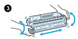
When toner is low, faded or light areas may appear on a printed page. You may be able to temporarily improve print quality by redistributing the toner. The following procedure may allow you to finish the current print job before replacing the toner cartridge.
