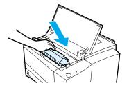
4 Reinsert the toner cartridge into the printer and close the top cover.
