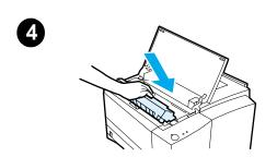
Over time, particles of toner and paper will begin to accumulate inside the printer. This may cause print quality problems during printing. Cleaning the printer will eliminate or reduce these problems.
