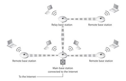
A main base station is connected to the Internet and shares its connection with remote and relay base stations. A remote base station shares the main base station's Internet connection. A relay base station shares the main base station's Internet connection and transfers the connection to other remote or relay base stations.
