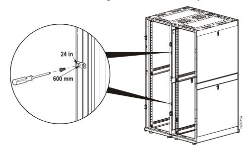
4. If 600-mm enclosures are joined together on 24-in centers, there is a gap between them. APC offers optional baying trim (AR7600) to cover the gap between the enclosures. The trim snaps into place without tools and can be installed after the units are joined together and have equipment installed in them.
