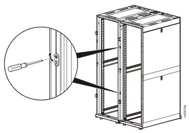
3. The 600-mm enclosures can be joined so that their centers are 24 in or 600 mm apart. Align the enclosures to use the appropriate holes on the front and rear of the enclosures for the spacing you need and secure the enclosures using one M5 x 12 flat-head screw per bracket.
