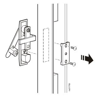
4. Remove the screw, latch, and washer from the back of the door handle assembly using the Torx T30/#2 Phillips wrench (provided). Rotate the washer 90 degrees and the latch 180 degrees and reattach the latch.
