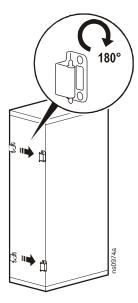
7. Remove the hinges from the door and reinstall them using the set of holes directly below where they were originally installed.
