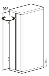
3. As you lift the door, turn it back to 60 degrees from the rack and lift the door off of its hinges to remove it.
