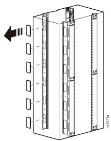
3. Reinstall the covers in the cable cutout holes on the rear vertical mounting flange of the air intake side of the enclosure.
