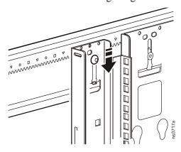
3. To align the vertical mounting flanges properly, note the symbol (for example, the diamond) visible through the one of the holes on the top of the flange, and ensure that the same symbol is visible through the corresponding hole at the bottom of the flange. Only one symbol is visible at a time through any of the holes. In the factory-standard position, the circles are visible through two of the holes.
